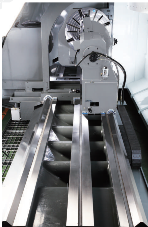
4 Bed Ways With Half Length Saddle
